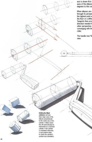
Start with a cylinder, of which the centre axis is drawn first as a guideline. The major axes of the ellipses are drawn at exactly 90 degrees to this centre axis.
