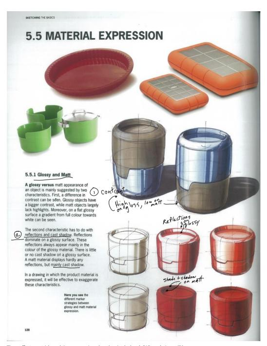
These effects are tricky and time-consuming when drawing by hand. CAD renderings will be more efficient if material surface information is really needed. But here's how to do it if you want to include the basics in your hand sketches.
